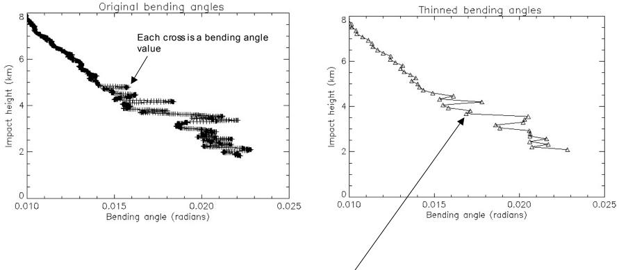
The bending angles we assimilate (triangles) are evaluated by interpolating the full resolution data to a set of fixed impact heights.
